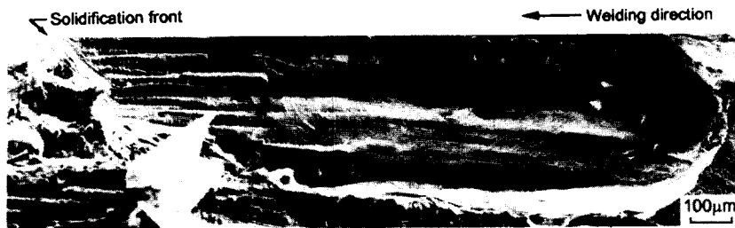
Photo. 3 Microfractograph of solidification crack in DS100 weld metal
