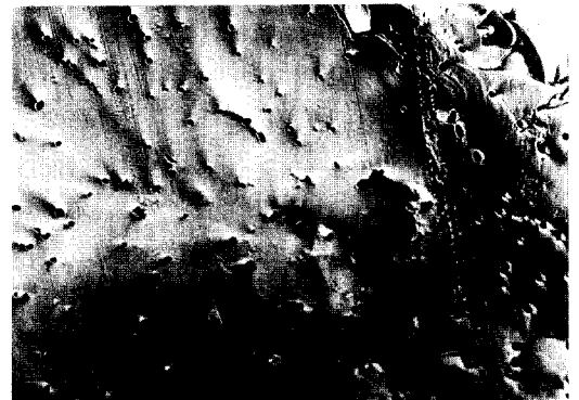
Fig. 7. Typical micropipes were observed under optical microscope on the surface of as grown 6H-SiC.
