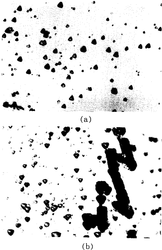
Fig. 5. The etch hillock pattern on the negative c-plane (a) etched for 1 minute and (b) etched for 2 minutes.
