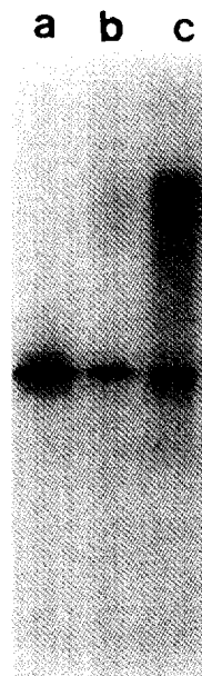
Fig. 4. Native PAGE analysis of laccase isozymes. a, hyphal tip laccase of dikaryon; b, secreted laccase of CL 110 in pH 4.2 medium; c, secreted laccase of CL 110 in pH 7.0 medium.
