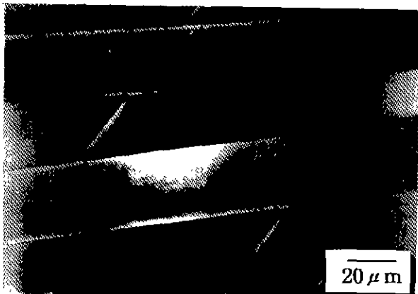
Fig. 1. SEM micrograph of 30ZrO_2 \cdot SiO_2 glass fibers heated at 800°C.
