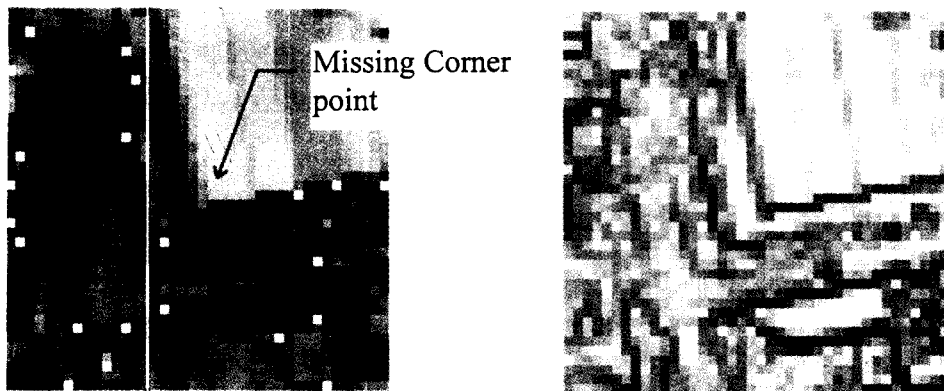
Fig. 9. Image patch and corresponding gradient image containing an undetected corner points caused by gradient disturbance.
