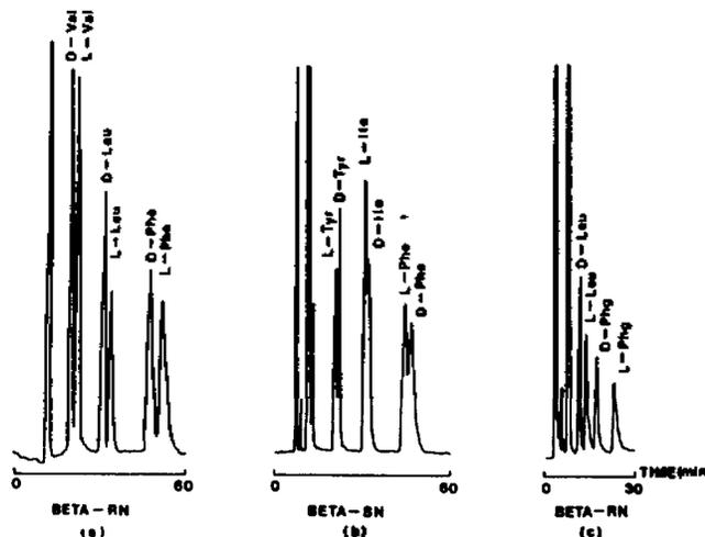
**Figure 1.** Chromatograms of DNP-(a), DNS-(b), DNB-Amino Acids(c) enantiomers on derivatized  $\beta$ -Cyclodextrin columns. Mobile Phase condition a) 50% MeOH : 50% Buffer Solution (0.5% TEA, pH 5.5). b) 20% MeCN : 80% Buffer Solution (0.7% TEA, pH 4.5). c) 50% MeOH : 50% Buffer Solution (0.7% TEA, pH 5.8) Flow Rate 1.0 mL/min.
