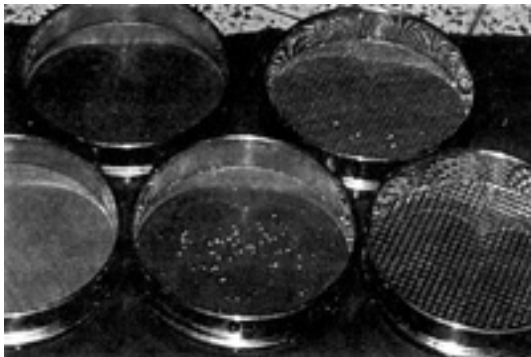
Fig. 7. Sieve system used in this study
