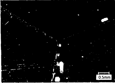
Fig. 2. Optical micrograph of the needle-shaped internal scattering defects (on the growth direction).
