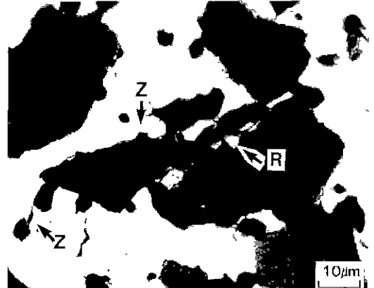
Fig. 2. Microstructure of the 20TiC-74Cr 3 C 2 -6ZrC specimen heat-treated at 1550°C for 15 min.
