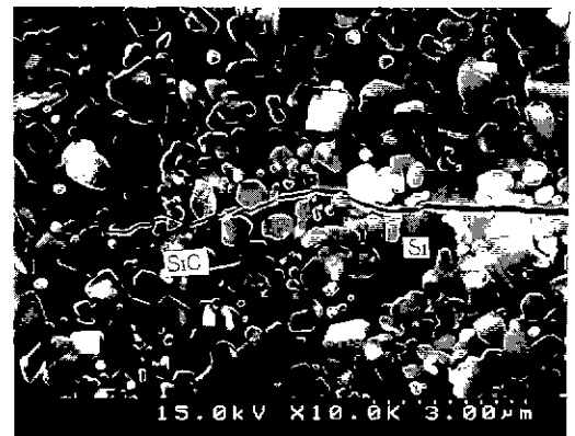
Fig. 7. SEM microstructure of reaction bonded SiC showing crack propagation
