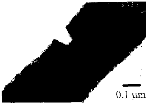
Fig. 6. Transmission electron micrograph of SiC whisker heat-treated after coating reaction.
