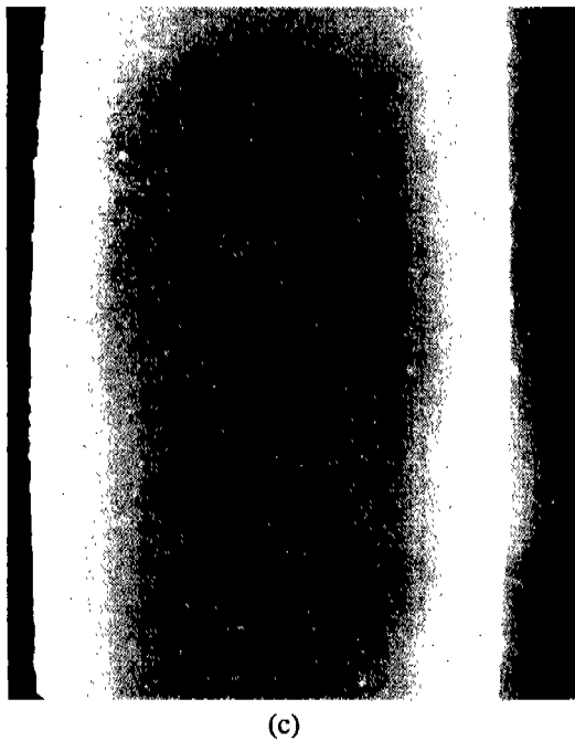
Fig. 7. Photomicrographs of PET POYs treated with water. (×1500) a: 60°C b: 80°C c: 100°C
