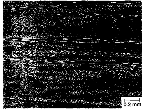
Fig.7 Photomicrograph of out-of-plane section through the chopped glass fiber/polyester resin SMC showing fiber bundles and voids
