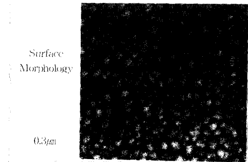
Fig. 7. The surface morphology of TiN substrate with Pd-HF activation pretreatment. (pretreat. time : 3min)
