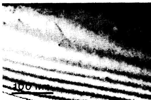
Fig. 2. Cross-sectional TEM micrograph of silicon surface etched using Ar plasma.
