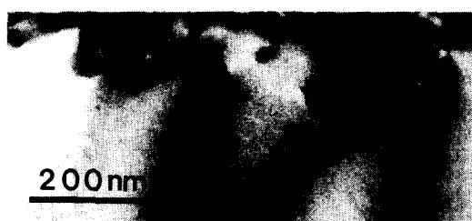
Fig. 6. Cross-sectional TEM micrograph of silicon surface annealed at 800°C for 30min after Ar/H<sub>2</sub> plasma etching.
