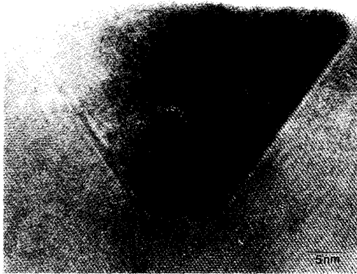
Fig. 7. HREM image of the Co/Ti bilayer annealed at 500°C, which shows a nucleus of CoSi 2 with coherent interface with Si substrate.
