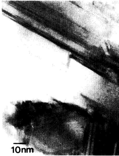
Fig. 6. TEM micrograph of twin boundary formed V shape.
