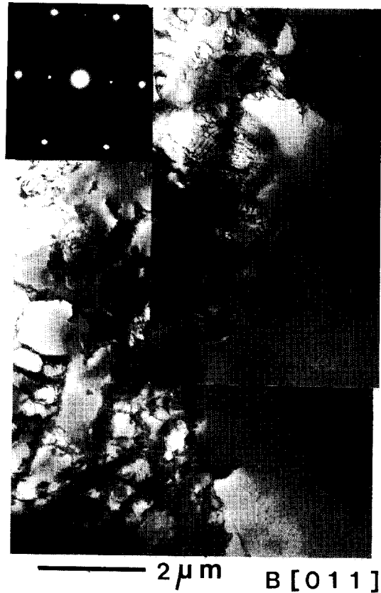
Fig. 8. TEM image and diffraction pattern between E2 and M1 area (Fig. 5) of SC blade
