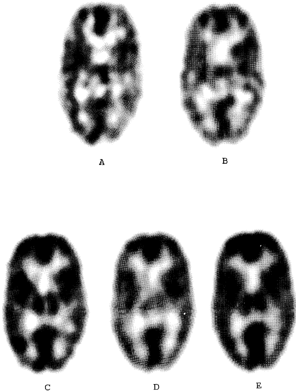
Fig. 9. The effects of noise in 3-D Hoffman brain phantom. The data were obtained for 1 min(A), 2min(B), 5min(C), 10min(D) and 20min(E). Each image used its own color scale for display purpose.
