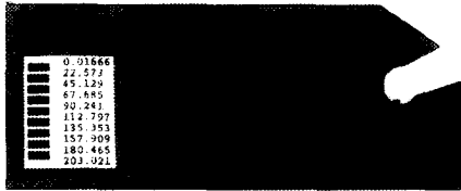
Fig. 3(a) Nodal stress solution of WC blade holder
