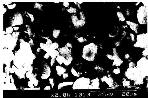
Fig. 1 SEM micrograph of the fine(5 \mu\text{m} ) \text{Al}_2\text{O}_3 powder.
