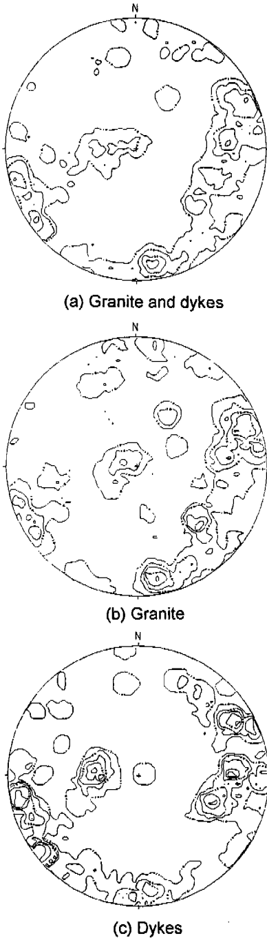
Fig. 4. Stereographic pole plots of the fractures measured from the study area (lower hemisphere).
