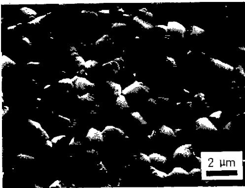
Fig. 6. SEM photograph of La(Mg 1/2 Ti 1/2 )O 3 specimen sintered at 1650°C
