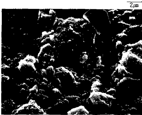
Fig.10 SEM Micrograph of 4 Cycle Aged Catalyst with H 2 O
