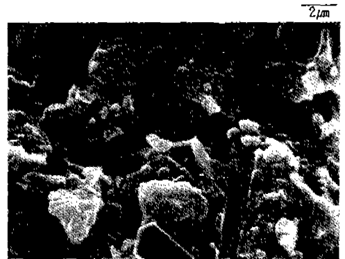
Fig.9 SEM Micrograph of 2 Cycle Aged Catalyst with H 2 O
