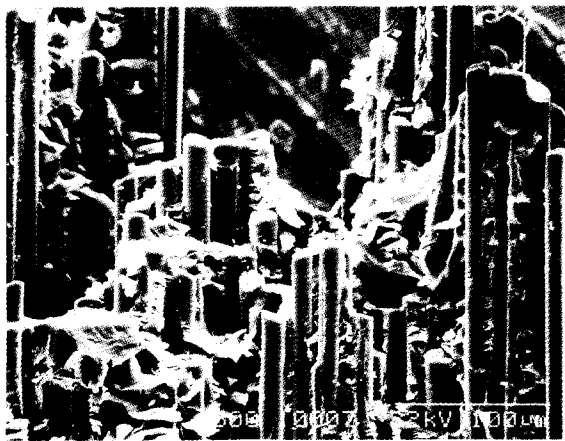
(b) 18µm sized glass fiber/epoxy composites(×300)
