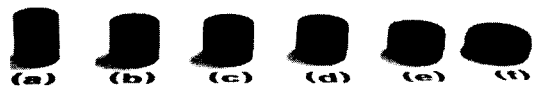
Fig.1 Experimental results for upsetting (a) initial billet (b) H.R.=15% (c) H.R.=20% (d) H.R.=25% (e) H.R.=40% (f) H.R.=60%
