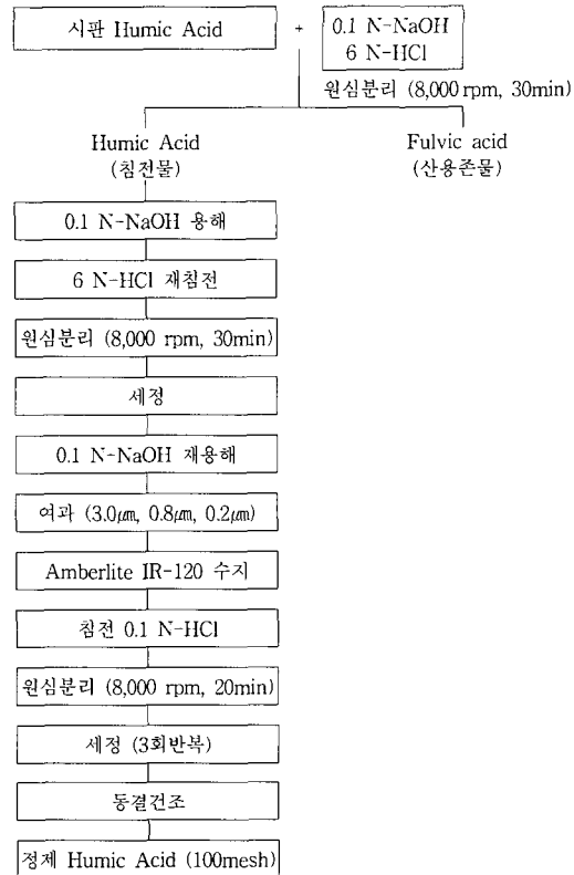
Scheme 1. Extraction and purification procedure of humic acid.
