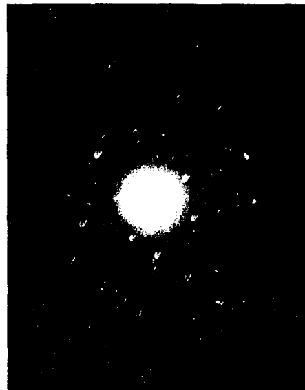
Fig. 4. Laue back reflection pattern of the grown ruby single crystal in [10\bar{1}0] direction.
