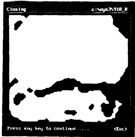
Fig. 3 The image resulting after applying the smoothing and closing process on the thresholded image in Fig. 2.
