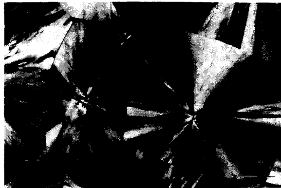
Figure 6. A polarizing optical micrograph (43 \mu\text{m} scale bar) of PTMS spherulites grown at 100 °C.
