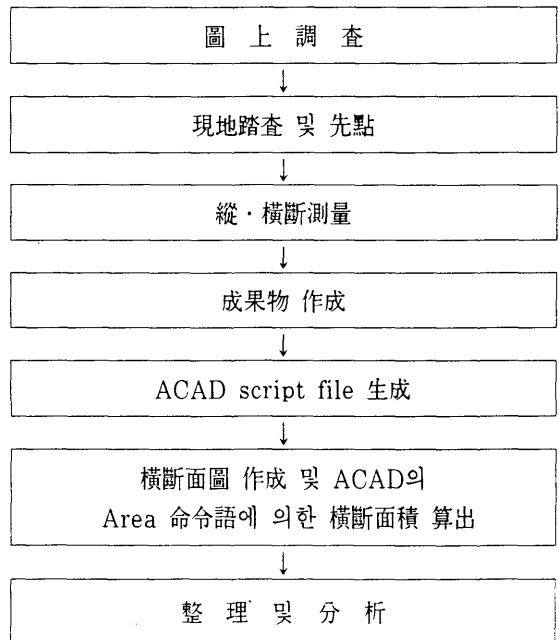
Fig. 3. The flow chart for river surveying and grasping channelbed fluctuation against urban river.
