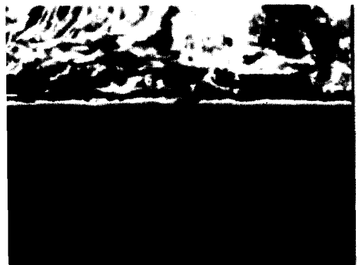
Fig. 11 Initiation of IGSCC of Inconel 600MA
