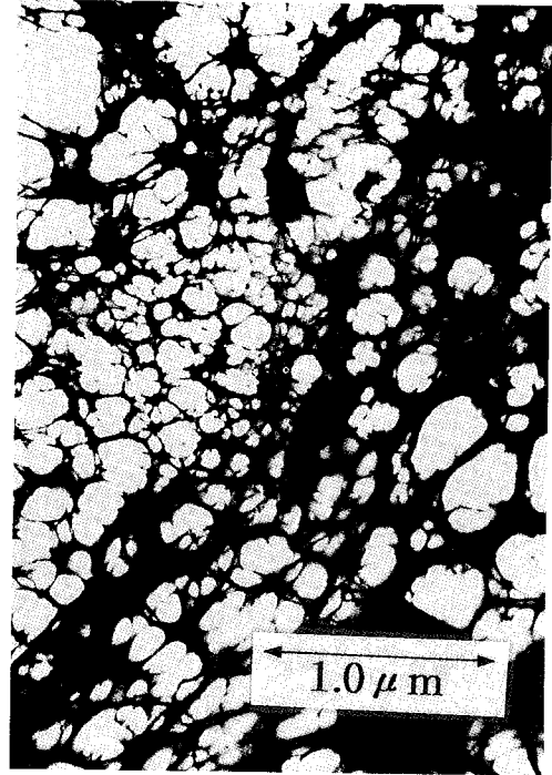
Fig. 10. Transmission electron micrograph of hydrophilic-hydrophobic polymer composite. This composite was prepared synthesizing the concentrated emulsion which was prepared by employing aqueous acrylamide solution as dispersed phase, styrene as continuous phase, and Span 80(0.25 mol/l styrene) as surfactant. The amount of the dispersed phase was 30g(2g acrylamide/28g water) and that of the continuous phase 5g (4g of styrene and 1 g of divinylbenzene). The initiator of dispersed phase was potassium persulfate(0.01g/g acrylamide) and that of continuous phase AIBN(0.01g/g styrene).
