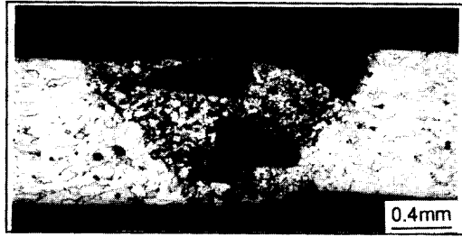
Fig. 13 An example of blow hole defects in the weld microstructure
