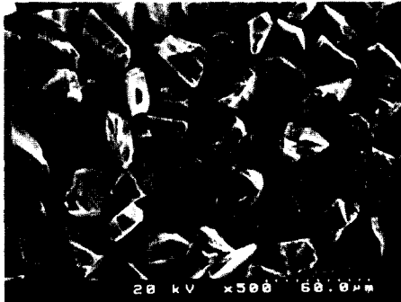
Fig. 9 Polygonal shape of diamond powders with the size of 20~30 μm.
