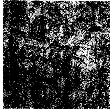
Fig. 9 An optical micrograph of an etched cross section of a specimen tested to rupture under an applied uniaxial tensile stress of 60 MPa. The stress direction is parallel to the vertical edge of this micrograph.
