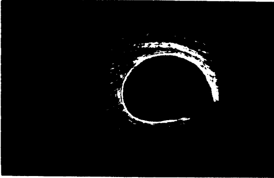
(b) K_{III} = 0.2763 (\text{Mpa} \cdot \text{mm}^{1/2}) Y_{\max} = 38.5 \text{mm} Z_i = 37 \text{mm} Z_0 = 680 \text{mm} \lambda = 19.3783
