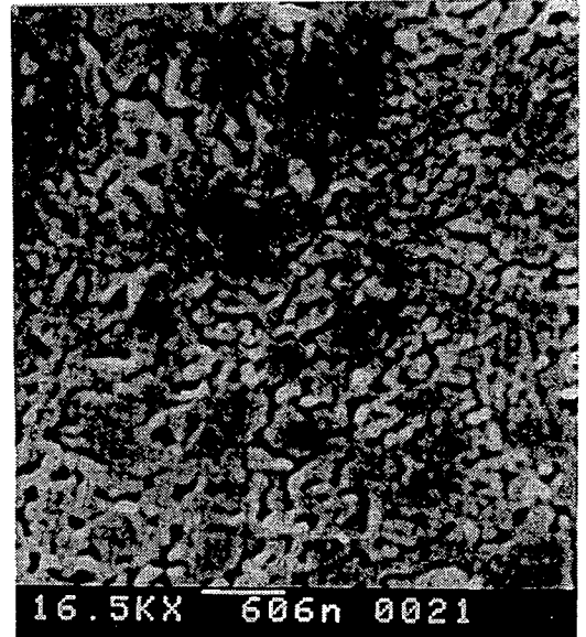
Fig. 9. Microstructure of glass ceramics surface perpendicular to pulling direction.
