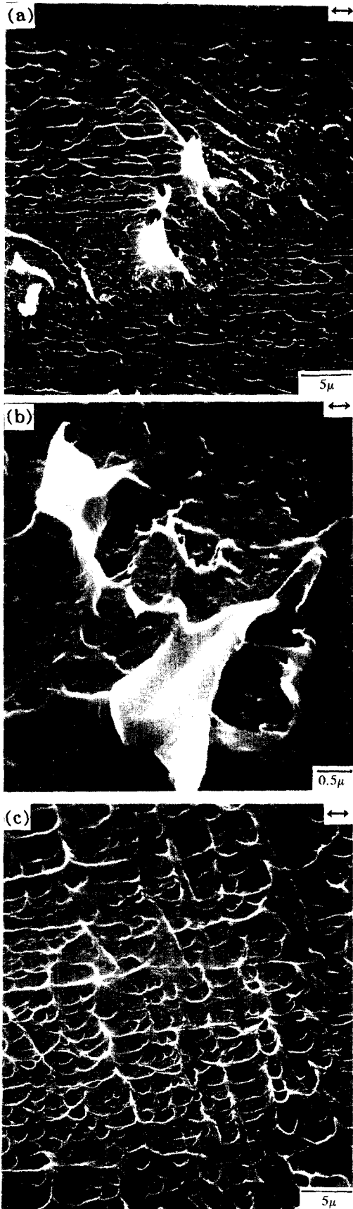
Fig. 13. SEM micrographs of the fracture surfaces bonded at 270°C under the pressure of 17 psi (a), (b) for 1 hour (c) for 10 hours
