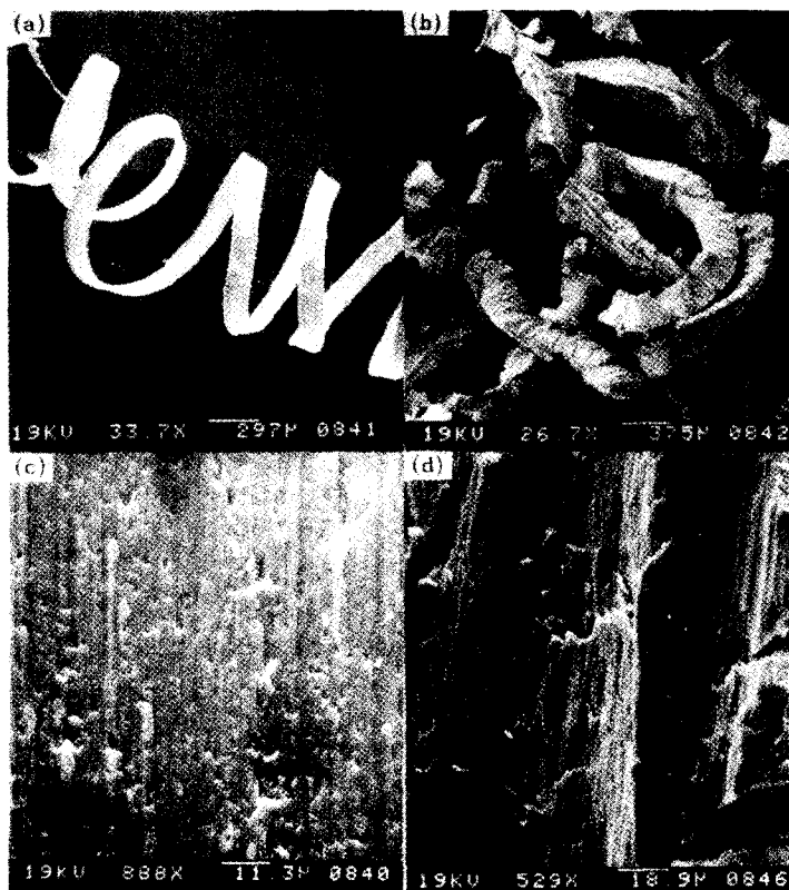
Photo. 4. Typical chips morphologies and fracture surface in the P/M 2011 Al alloys by SEM. ( f=0.014, d=0.1, \nu=84.7 )
