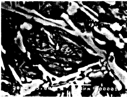
Fig. 7. Graphite nucleation at Fe 3 C and ferrite interface by decomposition of Fe 3 C. (a) simulation diagram (b) microstructure
