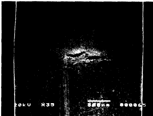
Fig. 15. Surface of the hump shoulder after CERT.
