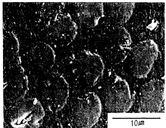
Fig. 7. SEM Micrograph of Carbon-Epoxy Composite
