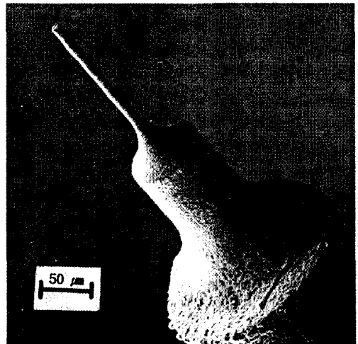
Fig. 8 Example of Machined Microshaft (Diameter 10μm, Length 300μm)
