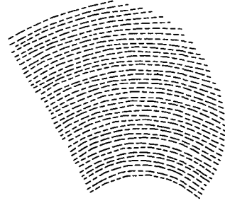
Fig. 11 Cutting tool path for a blade
