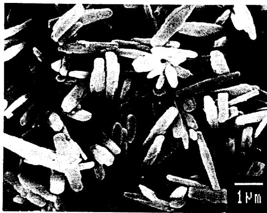
Figure 3. SEM photograph of \text{ZnGa}_2\text{O}_4:\text{Mn} phosphor prepared by the chemical method.
