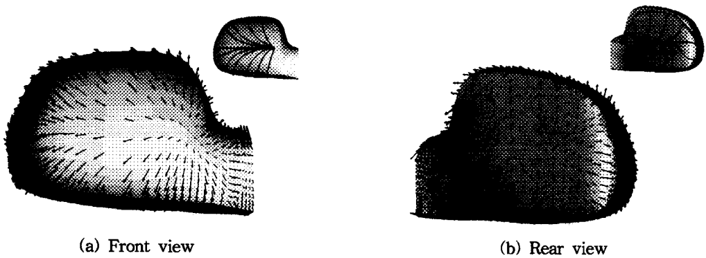
Fig.16 Velocity vectors and limiting streamlines on the side-view mirror
