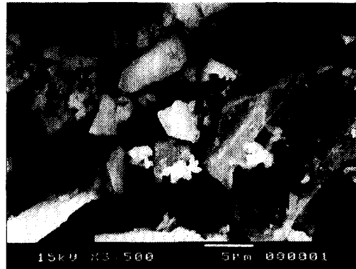
Fig. 8 Scanning electron micrograph of coal particles.
