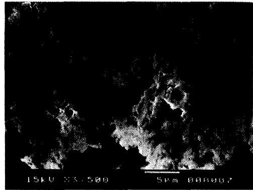
Fig. 9 Scanning electron micrograph of ash formed in the electric furnace.
