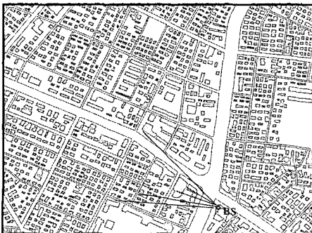
(Fig. 4) Signal prediction by building blockage loss
